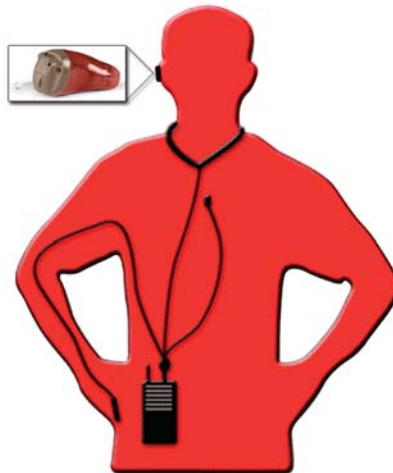
With a wireless induction loop and a receiving earpiece, you can completely camouflage your communications.
